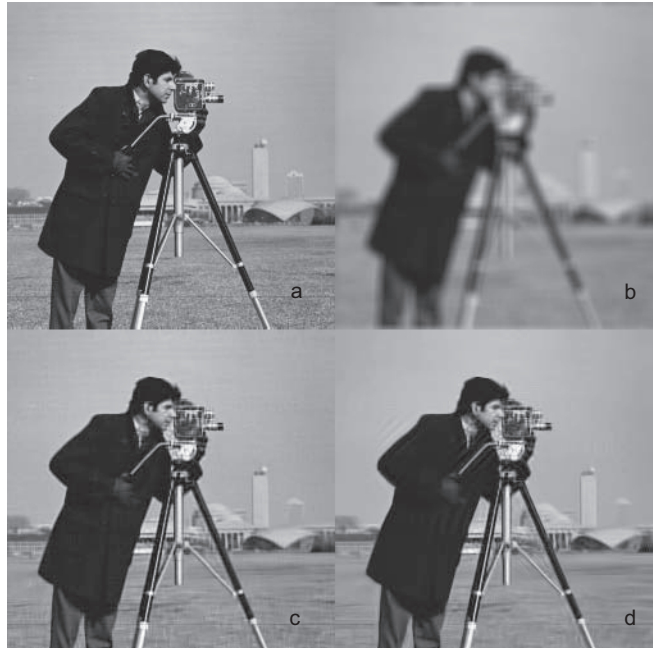
Figure 5. Cameraman test image: true (a), blurred noisy (b), DEB-NEM reconstruction after 20 iterations (c), DEBBM3D reconstruction (d).
