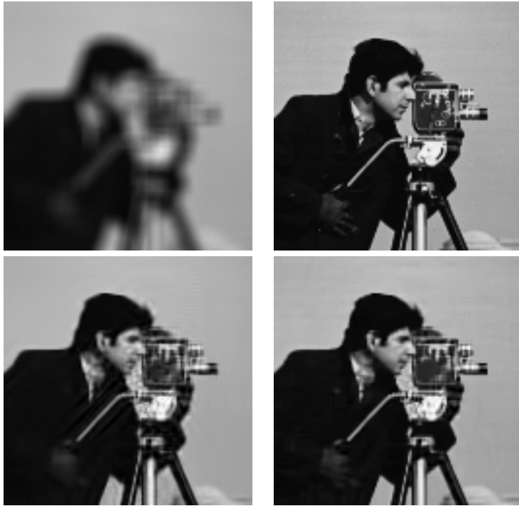
Figure 1. Deblurring experiment with the Cameraman image. From left to right and from top to bottom are presented zoomed fragments of the following images: blurred noisy, original, reconstructed by DEB-BM3D [3] and by proposed method.
