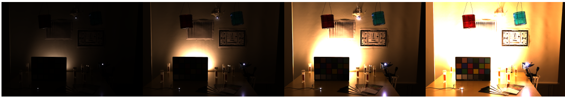
Figure 1.21: The four synthetic LDR frames used to create the HDR images shown tone mapped in the first row of 1.22. The exposure times used in creating the frames are 0.064, 0.256, 1.024, 4.096 seconds.
