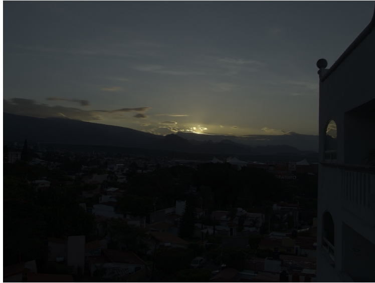
Figure 1.2: HDR image linearly scaled to fit the normal 8-bit display interval. The need for tone mapping is evident.
