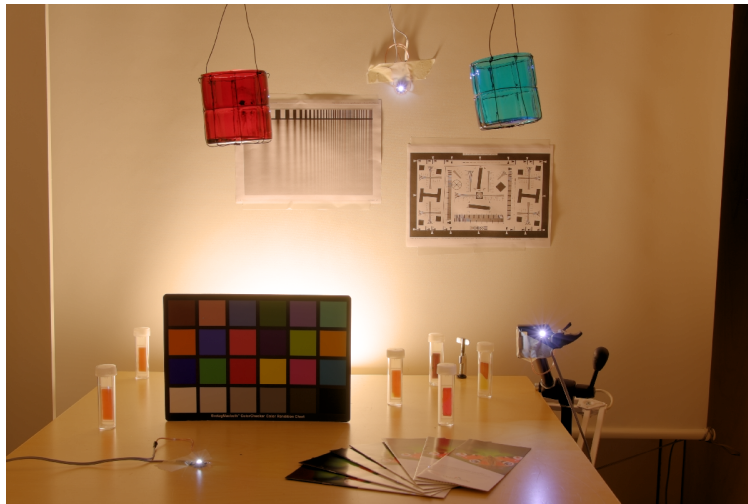
Figure 1.18: The HDR image composed in luminance-chrominance space from real data, tone mapped with the histogram adjustment technique presented in Section 1.5.2.
