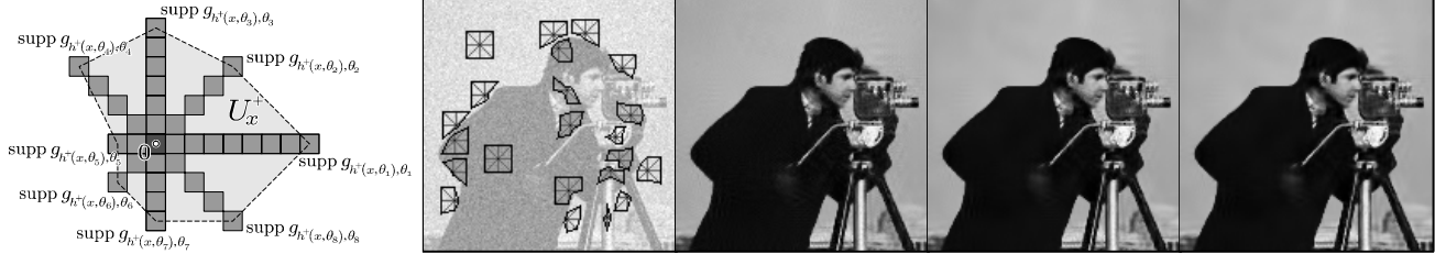
Figure 3. Fast implementation of the LPA-ICI anisotropic neighborhoods. “Linewise” one-dimensional directional LPA kernels are used for 8 directions. The anisotropic neighborhood U_x^+ is constructed as the polygonal hull of the adaptive-scale kernels’ supports (left). Some examples of the anisotropic neighborhoods \tilde{U}_x^+ used for SA-DCT filtering of the noisy Cameraman image (right), \sigma=25 . Only the adaptive scales h^+ are needed to construct the neighborhoods. The corresponding Anisotropic LPA-ICI SA-DCT hard-thresholding estimate \hat{y} (7) and Wiener estimate \hat{y}^{\text{wi}} (12), and Gilge’s “shape-adapted” DCT Wiener estimate ( PSNR =28.87, 29.10 dB, and 29.22 dB, respectively). In all the examples h=1,2,3,5,7,9 .
