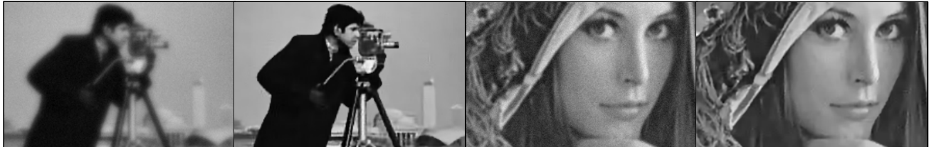
Figure 7. Fragments of the observations z and estimates \hat{g}^{RWI} for the deblurring experiments 3 and 4 ( ISNR=6.34 and 4.55 dB, respectively) .
