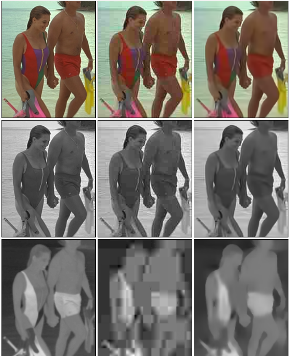
Figure 1.25: Fragments of the original, compressed, and restored Kodak image 12 . Top to bottom row: RGB color, luminance Y channel, chrominance V channel. From left to right: original image, JPEG-compressed ( Q=16 , 0.25bpp, PSNR=30.45dB), restored by proposed Pointwise SA-DCT method (PSNR=31.45dB).
