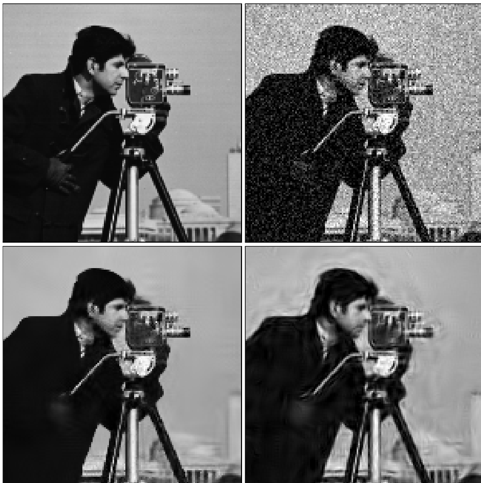
Figure 1.11: A fragment of Cameraman . Clockwise, from top-left: original, noisy observation ( \sigma=25 , PSNR=20.14dB), BLS-GSM estimate [138] (PSNR=28.35dB), and the proposed Pointwise SA-DCT estimate (PSNR=29.11dB).
