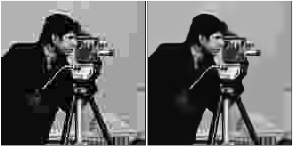
Figure 1.14: Details of the JPEG-compressed Cameraman ( Q=6 , \text{bpp}=0.19 , \text{PSNR}=25.03\text{dB} ) and of the corresponding Pointwise SA-DCT estimate ( \text{PSNR}=26.11\text{dB} ). The estimated standard deviation for this highly compressed image is \sigma=17.6 .
