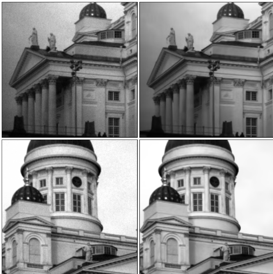
Figure C.5: Fragments of raw-data from CMOS sensor before and after Pointwise SA-DCT denoising with noise parameters estimated automatically.
