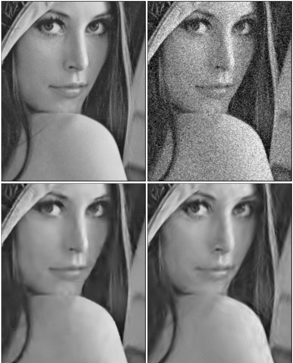
Figure 1.10: A fragment of Lena . Clockwise, from top-left: original, noisy observation ( \sigma=25 , PSNR=20.18dB), BLS-GSM estimate [138] (PSNR=31.69dB), and the proposed Pointwise SA-DCT estimate (PSNR=31.66).
