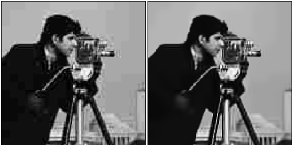
Figure 1.15: Details of the JPEG-compressed Cameraman ( Q=15 , \text{bpp}=0.37 , \text{PSNR}=27.71\text{dB} ) and of the corresponding Pointwise SA-DCT estimate ( \text{PSNR}=28.58\text{dB} ). The estimated standard deviation for this compressed image is \sigma=9.7 .
