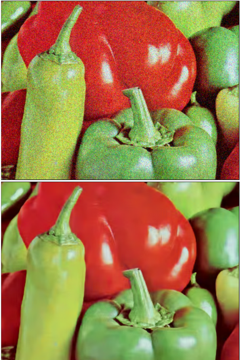
Figure 1.21: Fragments from the noisy ( \sigma=25 , PSNR=20.18dB) and denoised color Peppers image (PSNR=30.90dB), obtained using the proposed Pointwise SA-DCT algorithm.
