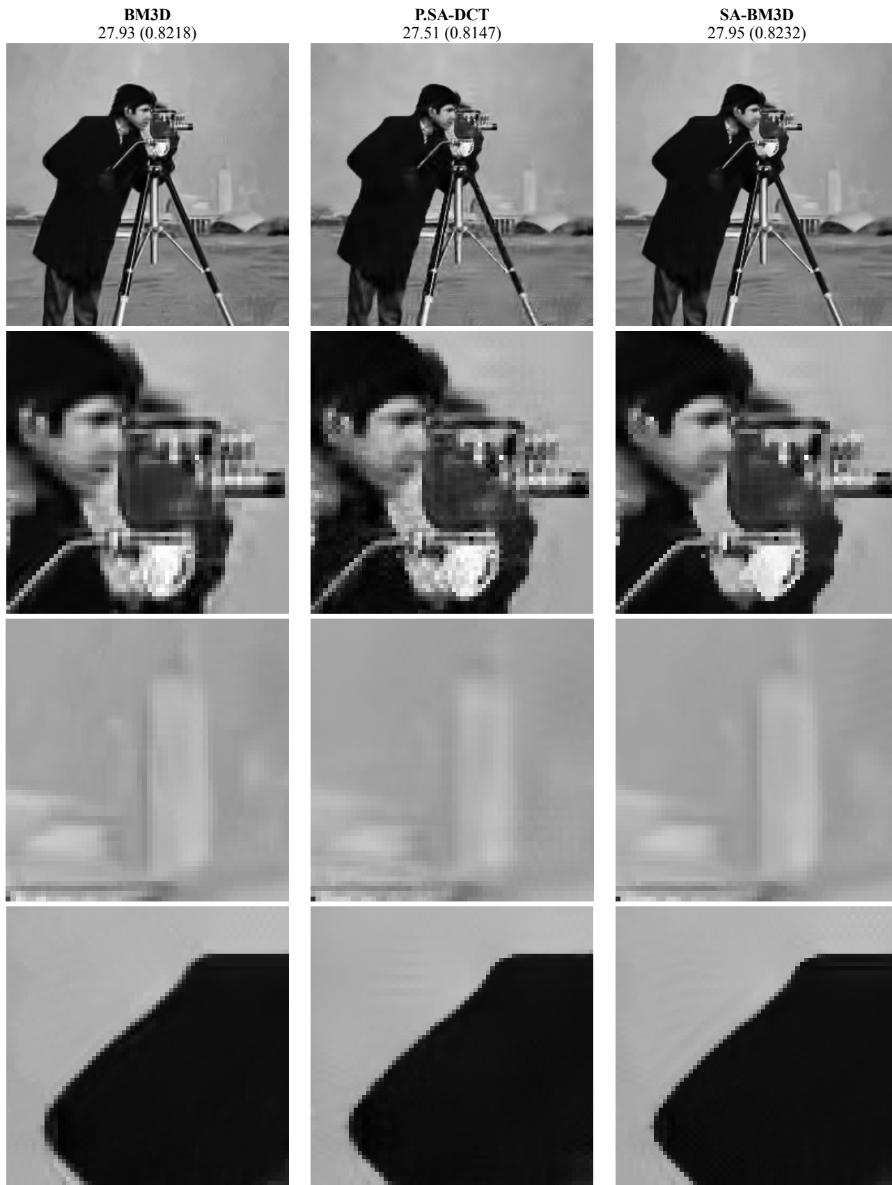
Figure 6: Comparison between denoised Cameraman by the BM3D (left), the SA-DCT (center), and the SA-BM3D (right) filters. The numbers above the images are the corresponding PSNR and SSIM (in parentheses) values (calculated on the whole image). The standard deviation of the noise in the input image is \sigma = 35 .
