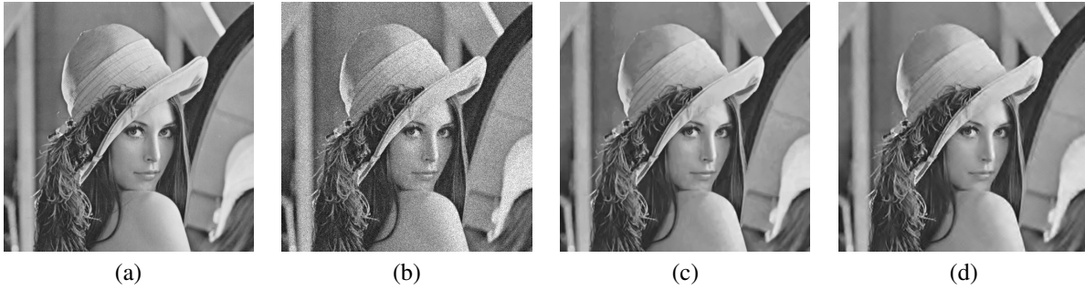
Fig. 7. The denoising of Lena ( 512 \times 512 ). (a) Original image, (b) Noisy image (peak = 100, \sigma = 2 , PSNR = 22.64 dB), (c) Denoised with BM3D and the exact unbiased inverse \mathcal{I}_\sigma (PSNR = 33.41 dB), (d) Denoised with UWT/BDCT PURE-LET (PSNR = 32.92 dB).
