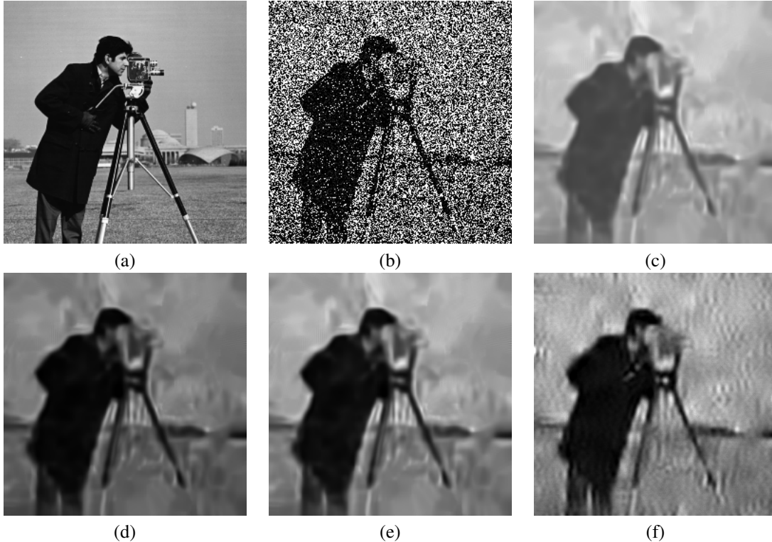
Fig. 9. The denoising of Cameraman ( 256 \times 256 ). (a) Original image, (b) Noisy image (peak = 1, \sigma = 0.1 , PSNR = 3.20 dB), (c) Denoised with BM3D and the asymptotically unbiased inverse \mathcal{I}_{\text{asy}} (PSNR = 15.55 dB), (d) Denoised with BM3D and the algebraic inverse \mathcal{I}_{\text{alg}} (PSNR = 15.72 dB), (e) Denoised with BM3D and the exact unbiased inverse \mathcal{I}_\sigma (PSNR = 20.23 dB), (f) Denoised with UWT/BDCT PURE-LET (PSNR = 20.35 dB).
