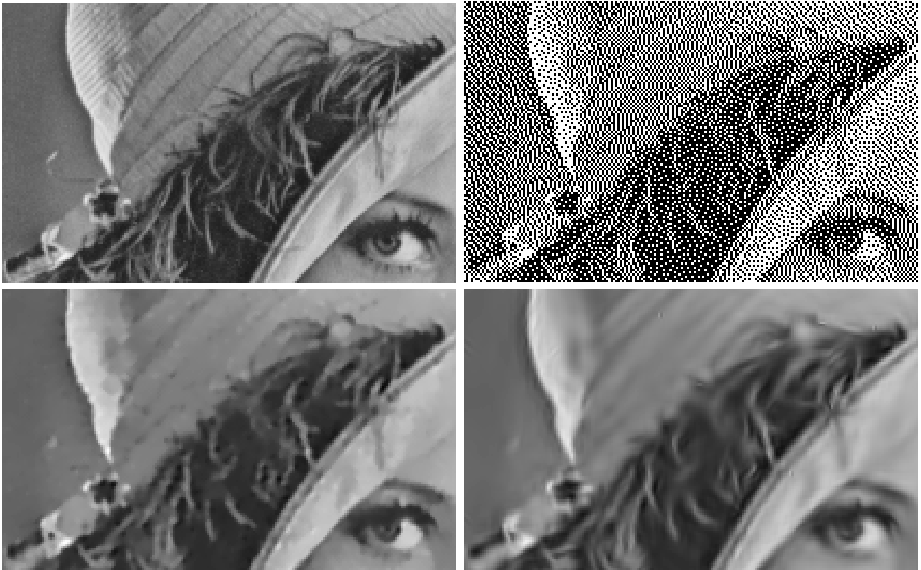
Figure 10: Visual comparison for a detail of the Lena image: from left to right, original and Floyd-Steinberg halftone (top), the proposed anisotropic LPA-ICI estimate ( PSNR=32.4 ), and the “ WInHD ” estimate [26] ( PSNR=32.1 ) based on deconvolution and filtering in the complex wavelet domain [17].
