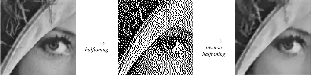
Figure 1: An illustration of halftoning and inverse halftoning. Detail of the Lena image: original (left), Jarvis error diffusion halftone (center), and LPA-ICI estimate ( PSNR=33.0dB ) (right).
