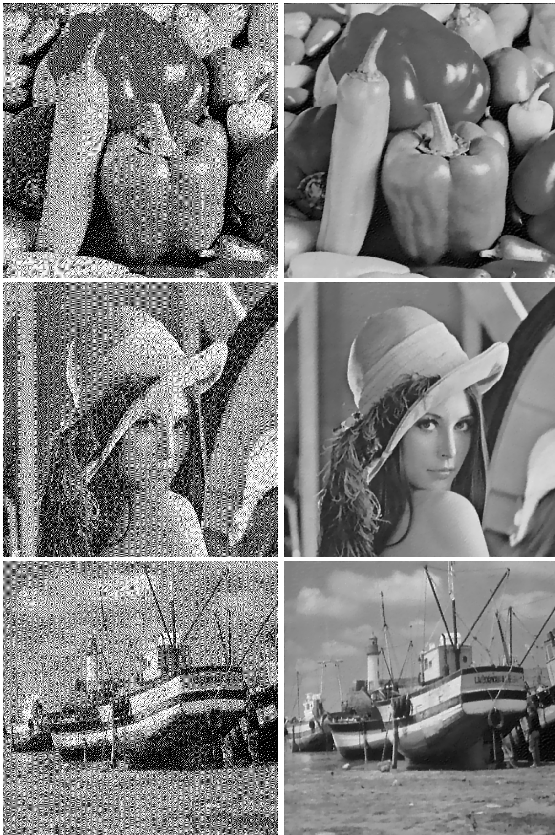
Figure 9: Examples of Floyd-Steinberg error diffusion LPA-ICI inverse halftoning: Peppers ( PSNR=31.6\text{dB} ), Lena ( PSNR=32.4\text{dB} ), and Boats ( PSNR=29.5\text{dB} ). The pictures in the right column are the estimates obtained by the proposed procedure from the binary halftone images (shown in the left column).
