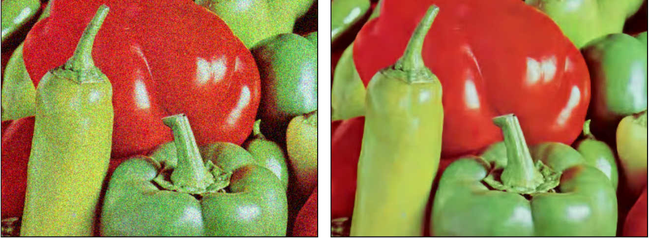
Fig. 4. Fragments from the noisy ( \sigma=25 , PSNR=20.18dB) and denoised Peppers image (PSNR=30.90dB), obtained using the proposed SA-DCT algorithm.
