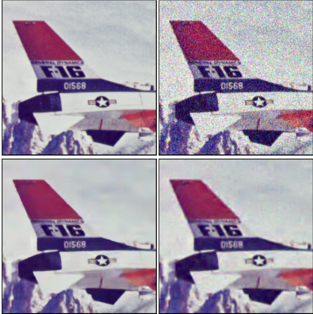
Fig. 3. Fragments of the original F-16 image (top-left), of its noisy observation ( \sigma=30 , PSNR=18.59) (top-right) and of two denoised estimates: our SA-DCT estimate (bottom-left), and the ProbShrink-MB [8] estimate (bottom-right). The PSNR for the two estimates is 31.59dB and 30.50dB, respectively.
