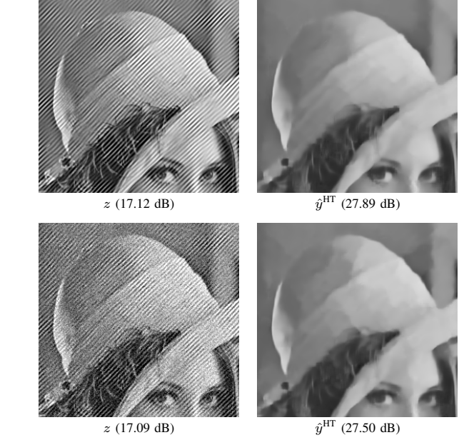
Figure 9. View of denoising of Lena corrupted by correlated noise defined by g_3 (top) and g_7 of (4) (bottom), both with \|g\|_2^2 = 0.02 . On left, the noisy images z , and on right the corresponding hard-thresholding estimates \hat{y}^{\text{HT}} .
