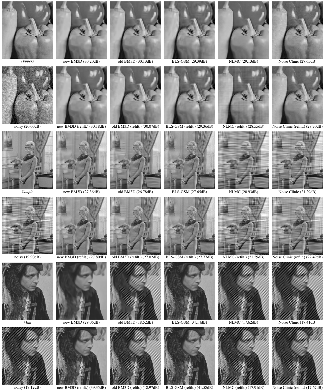
Figure 18. A view of Peppers with white noise (kernel g_w , \|g\|_2^2 = 0.01 ), Couple with horizontal noise (kernel g_1 , \|g\|_2^2 = 0.01 ), and Man with diagonal pattern noise (kernel g_3 , \|g\|_2^2 = 0.02 ). Denoising results of BM3D with the proposed improvements, old BM3D, BLS-GSM, NLM-C and Noise Clinic, as well as these methods with the applied refiltering procedure. Note how the new BM3D yields significant improvements compared to the old BM3D in both cases of correlated noise, while keeping the same performance in white noise. Refiltering restores visible details for both correlated noise cases, without affecting the performance for white noise. Furthermore, especially with the noise generated by g_3 , refiltering restores significant detail also for the BLS-GSM algorithm.
