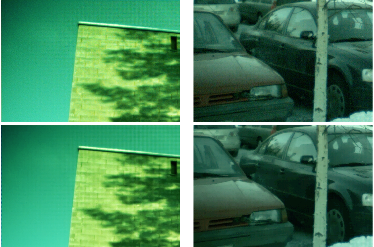
Figure 8. Fragments of images that illustrate the restoration of real noisy Bayer data measured directly from the sensor of a camera phone: (first row) Hamilton-Adams CFAI 7 ; (second row) proposed technique.
