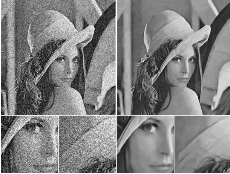
Figure 5. On the left are noisy ( \sigma = 35 ) Lena and two enlarged fragments from it; on the right are the denoised image (PSNR 30.61 dB) and the corresponding fragments.
