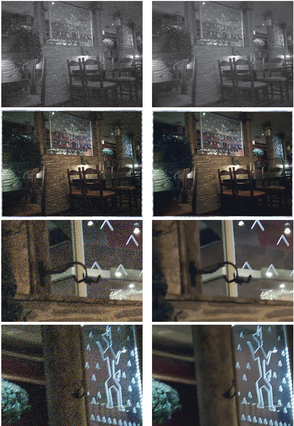
Figure 5.8: Results of applying the BM3D filter in conjunction with the variance stabilizing and declipping transformations from [Foi09] on a 5 MPix raw Bayer image taken in a dim environment using analog gain 16. The top row contains the G1 green channels (gamma corrected for better visibility) of the original and the denoised raw images; the second row contains RGB images obtained by applying an identical image processing chain both to the original and to the denoised raw images. In addition, the last two rows show enlarged fragments of these RGB images.
