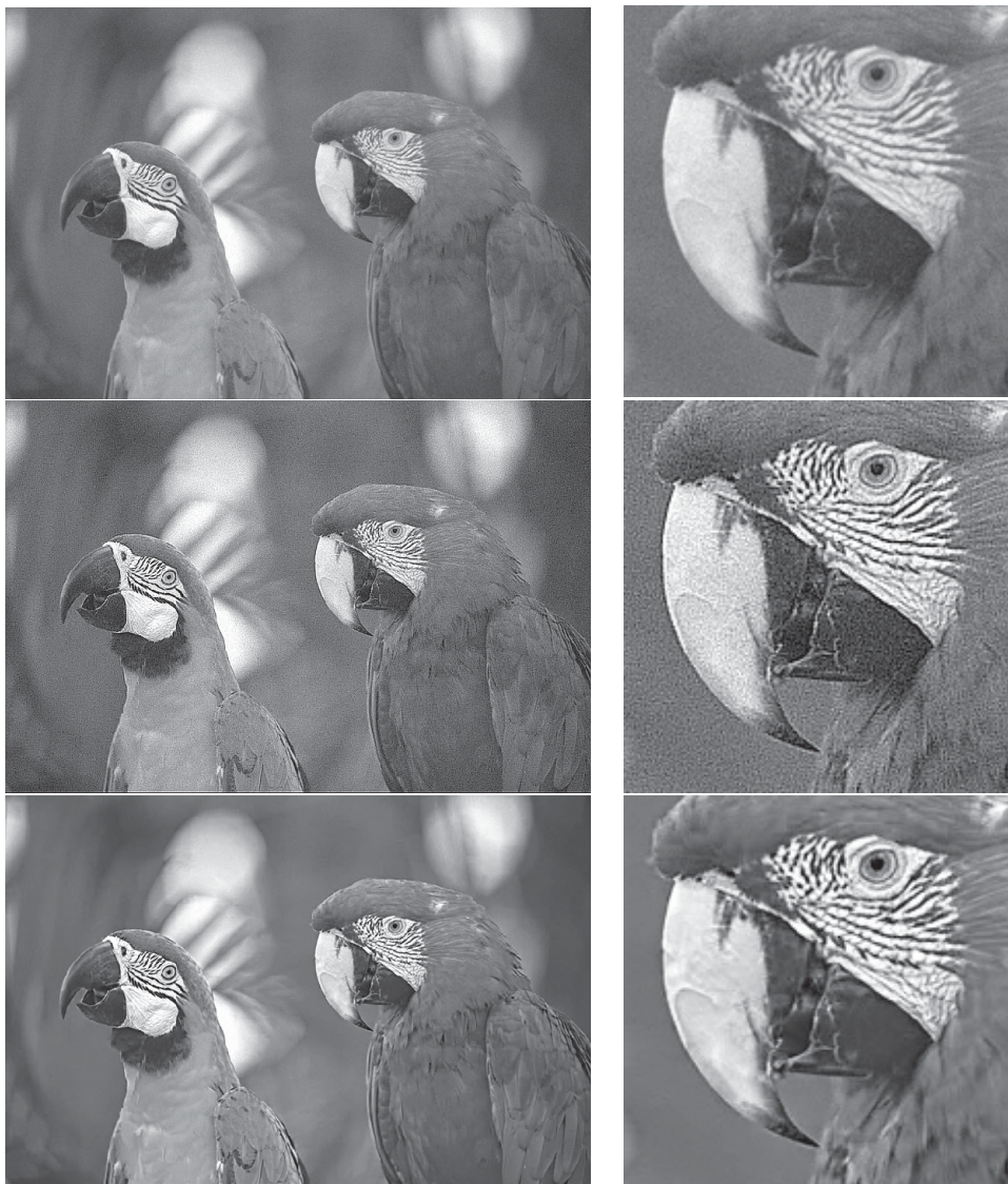
Figure 5.15: Illustration of image sharpening applied on the luminance of Kodak image 23 with quite mild AWGN (with \sigma=5 ); this image is given in the top along with an enlarged fragment of it. The second row is the result of applying the standard unsharp mask method; the original image is sharpened but there are notable noise amplification problems. The third row presents the result of the proposed method, which does not contain noise-amplification artifacts and the image appears sharpened.
