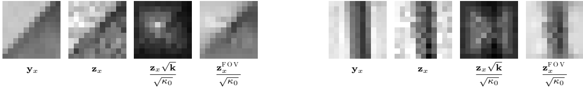
Figure 4. Two illustrative examples of how patches are transformed when computing the windowed distance d (4) and the foveated distance d^{\text{FOV}} (6): \mathbf{z}_x denotes the patch in the noisy image, while \mathbf{z}_x \sqrt{\mathbf{k}} and \mathbf{z}_x^{\text{FOV}} denote, respectively, the patches used for computing the quadratic windowed distance and foveated distance, for the same image and fixation point. The division by \sqrt{\kappa_0} ensures that these patches are displayed on the same intensity range of \mathbf{z}_x . In both examples the noise standard deviation in \mathbf{z}_x is \sigma = 20 and \mathbf{y}_x , the noise-free counterpart of \mathbf{z}_x , is also shown.
