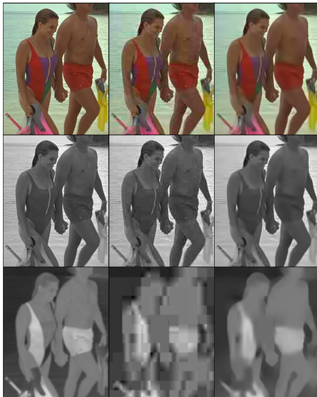
Figure 5: Fragments of the original, compressed, and restored Kodak image 12. Top to bottom row: RGB color, luminance Y channel, chrominance V channel. From left to right: original image, JPEG-compressed ( Q=16 , 0.25bpp, PSNR=30.45 ), restored by proposed Pointwise SA-DCT method ( PSNR=31.45 ).
