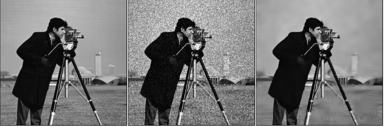
Figure 4: Cameraman image: (from left to right) original image, noisy observation corrupted by Poissonian noise ( \chi = 30/255 , MSE=1015, PSNR=18.1dB), and Pointwise Shape-Adaptive DCT estimate \hat{y}^{\text{wi}} (MSE=100, PSNR=28.1dB).
