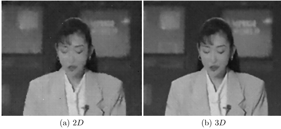
Figure 10.3: Frame 41 from the Akiyo sequence: (a) restored with 2D algorithm, (b) restored with the proposed 3D algorithm.
