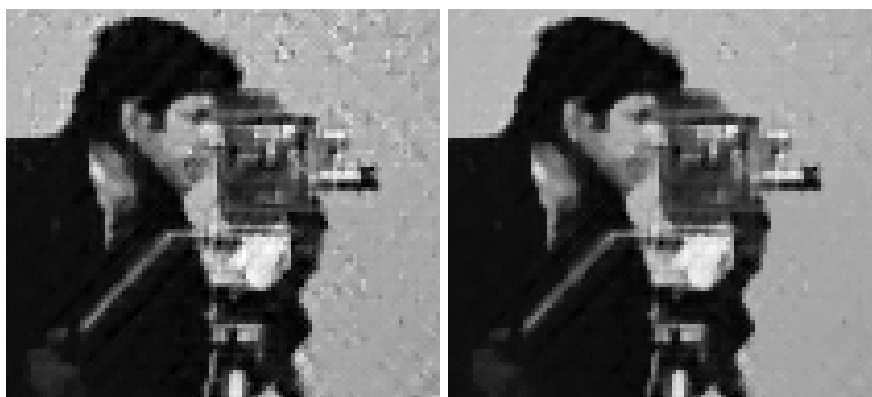
Figure 9.9: Filtering the Poisson data by the algorithm developed for the Gaussian one. Standard selection of the algorithm parameters gives a poor estimate, ISNR=5.38\text{dB} (left). Up to some extent, it can be improved by manually optimizing some algorithm parameters, ISNR=6.03\text{dB} (right).
