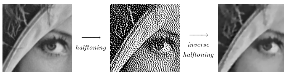
Figure 9.10: An illustration of halftoning and inverse halftoning. Detail of the Lena image: original (left), Jarvis error-diffusion halftone (center), and LPA-ICI estimate ( PSNR=33.0\text{dB} ) (right).
