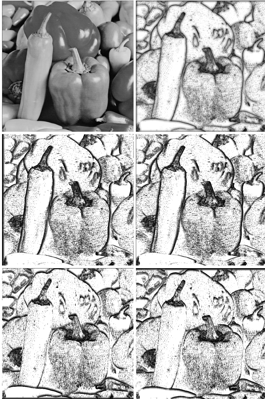
Figure 7.20: Peppers image (top left), adaptive scales for the horizontal (middle) and vertical (bottom) left derivative (left) and right derivative (right). The mean value of the adaptive scales computed among all directions is shown in the top right subimage. Observe how the adaptive scales reveal the edges and contours of the image.
