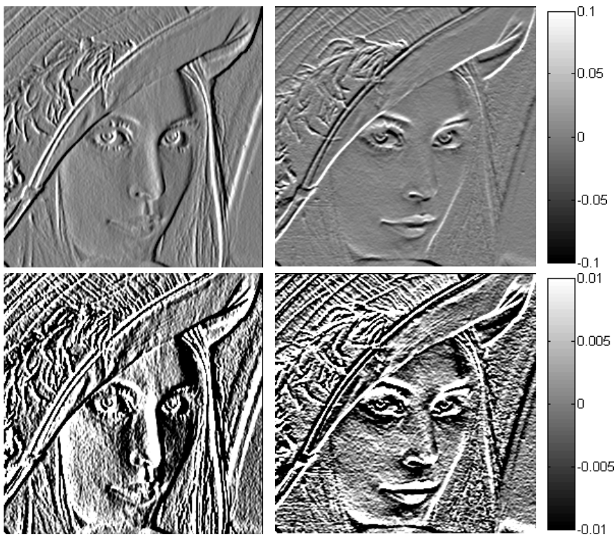
Figure 7.19: Sobel derivative filters: \frac{\partial f}{\partial x_1} (left column) and \frac{\partial f}{\partial x_2} (right column). Same results are shown in different rows with different contrast to enhance visualization.
