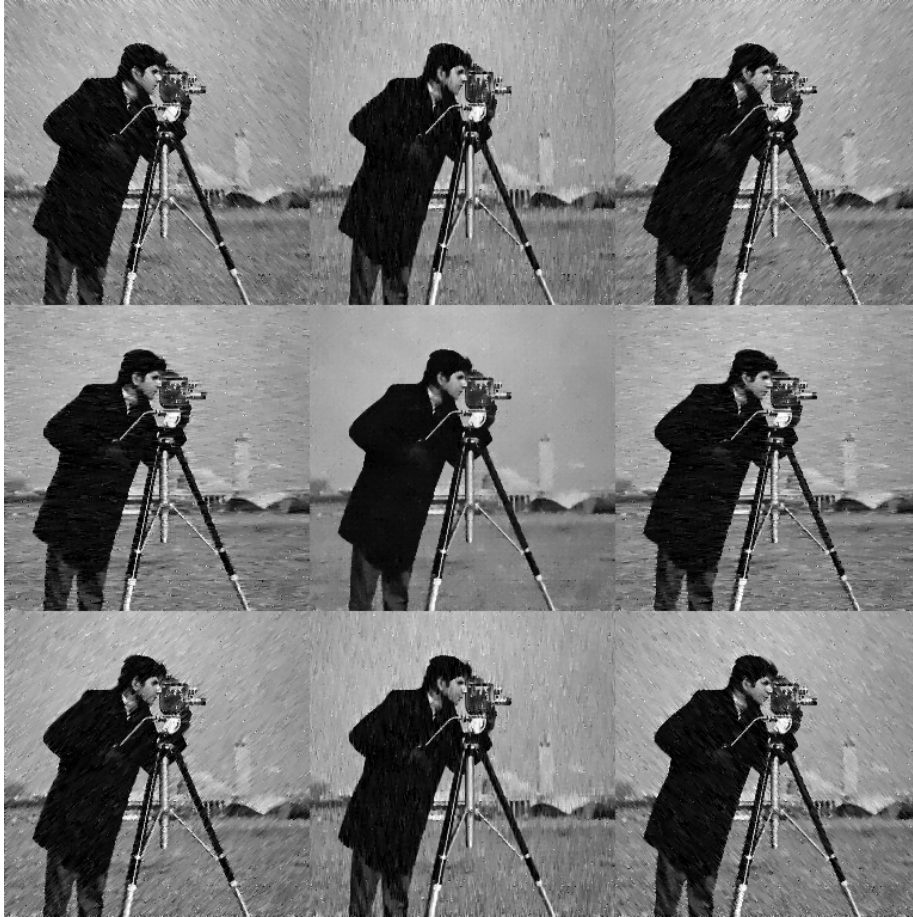
Figure 4.10: Clockwise from top-left, the adaptive-scale estimates \hat{y}_{h+(x,\theta_k)}(x) \forall x , \theta_k = \frac{7\pi}{4}, \frac{3\pi}{2}, \frac{5\pi}{4}, \pi, \frac{3\pi}{4}, \frac{\pi}{2}, \frac{\pi}{4}, 0 , and, in the center, the fused anisotropic estimate \hat{y} .
