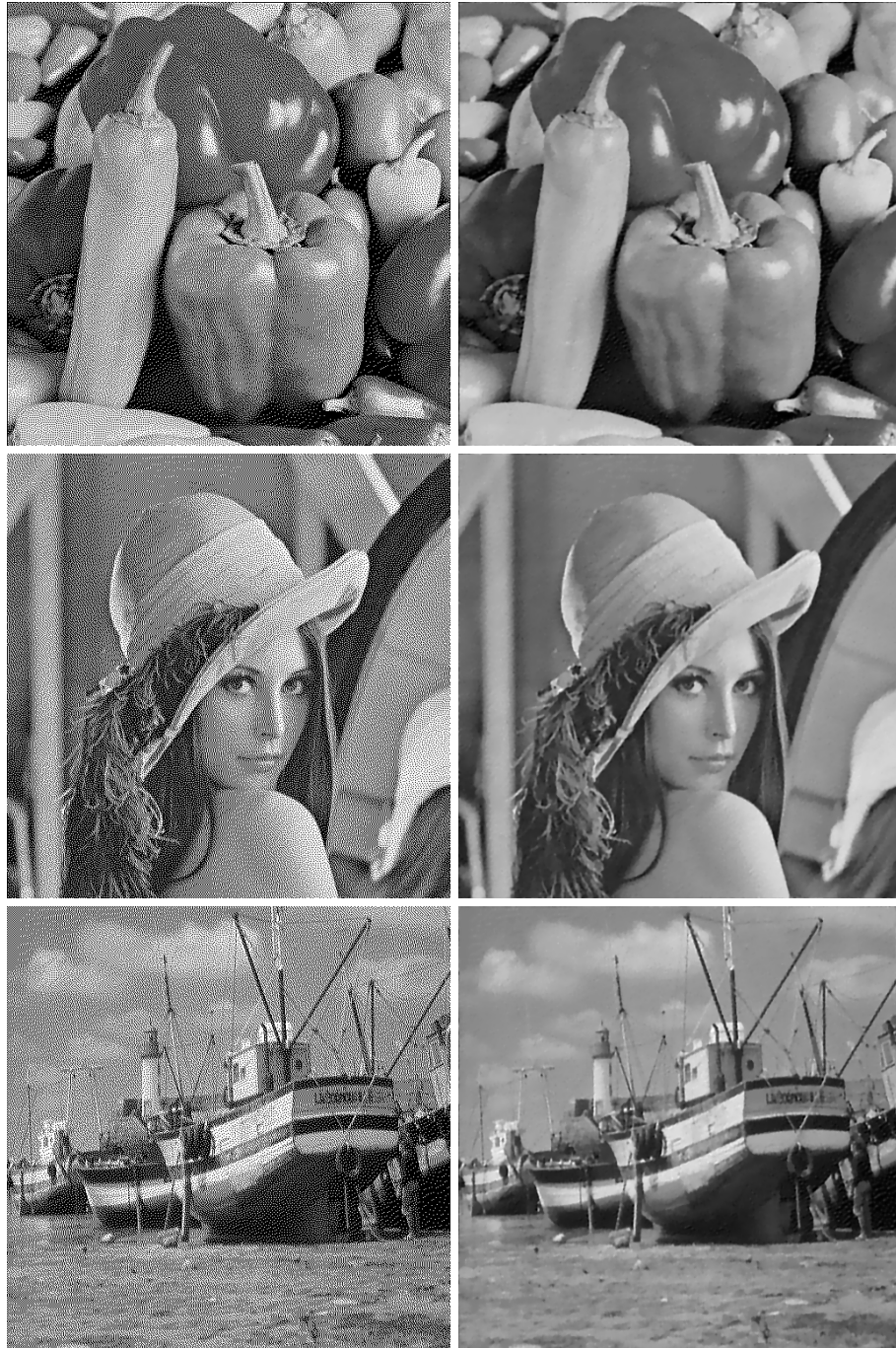
Figure 9.16: Examples of Floyd-Steinberg error diffusion LPA-ICI inverse halftoning: Peppers ( PSNR=31.6\text{dB} ), Lena ( PSNR=32.4\text{dB} ), and Boats ( PSNR=29.5\text{dB} ). The pictures in the right column are the estimates obtained by the proposed procedure from the binary halftone images (shown in the left column).
