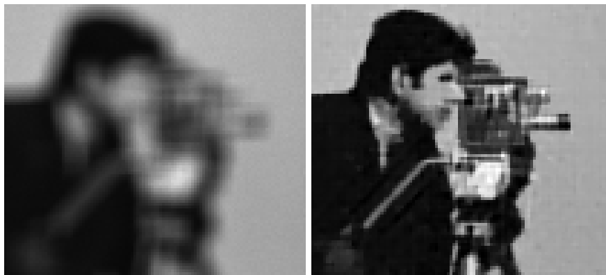
Figure 9.6: Deblurring the Cameraman image. Left is a fragment of the noisy blurred observation ( BSNR=32.5\text{dB} ). Right is the reconstructed image obtained by the proposed Poissonian adaptive deconvolution algorithm, ISNR=6.61\text{dB} .
