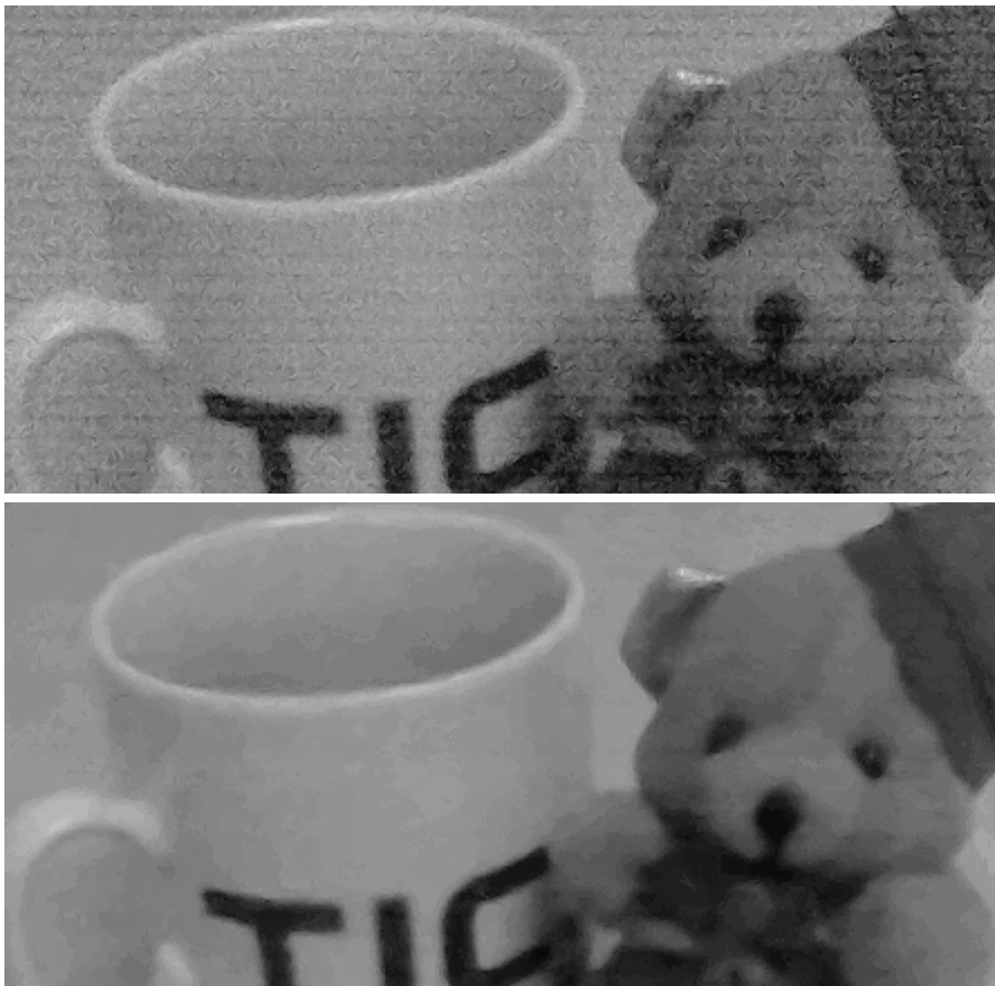
Figure 8.13: Color image reconstructed, using the standard imaging chain, from the noisy raw data (top) and from the LPA-ICI -filtered raw data (bottom).
