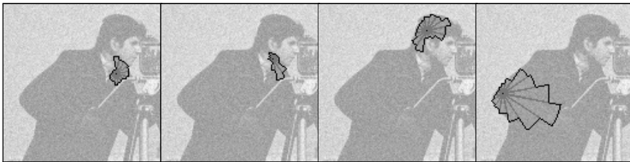
Figure 4.4: Cameraman (detail): adaptive anisotropic neighborhoods \tilde{U}_x^+ obtained through ICI using sectorial kernels
