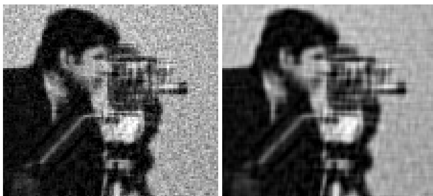
Figure 9.7: Result of the pure regularized inverse z^{RI} from (9.6) (left) and the “oracle” Wiener estimate, ISNR=5.22\text{dB} (right).
