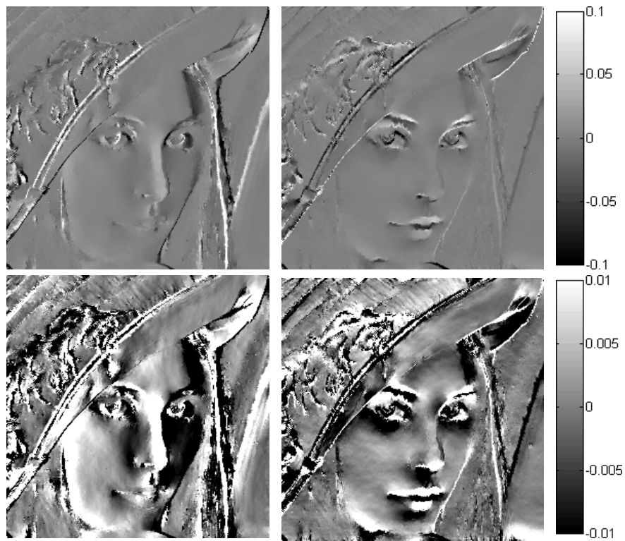
Figure 7.18: Anisotropic gradient: \frac{\partial f}{\partial x_1} (left column) and \frac{\partial f}{\partial x_2} (right column). Same results are shown in different rows with different contrast to enhance visualization.
