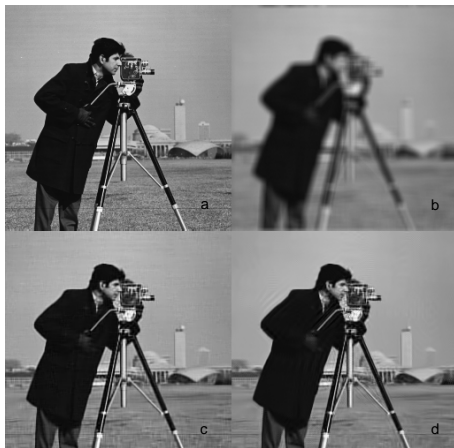
Cameramen test image: true (a), blurred noisy (b), DEB-NEM reconstruction after 20 iterations (c), DEBBM3D reconstruction (d).
