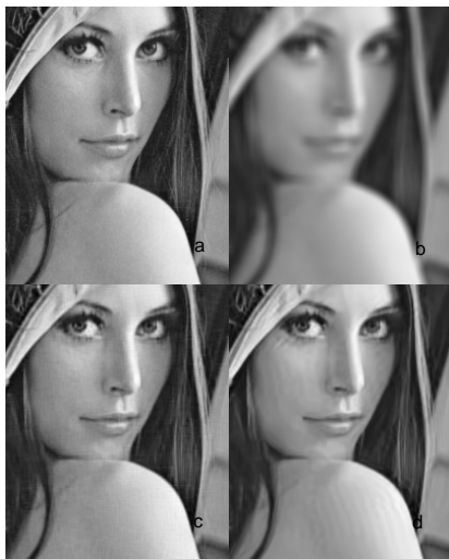
A fragment of Lena test image: true (a), blurred noisy (b), DEB-NEM reconstruction after 20 iterations (c), DEBBM3D reconstruction (d).
