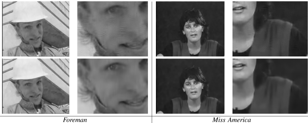
Fig. 13. Denoising results for Foreman and Miss America corrupted by synthetic correlated noise having \varsigma_{\text{RND}} = \varsigma_{\text{FPN}} = 15 using E-RF3D to separately remove the two noise components. Top: first suppression of random noise and then FPN ( Foreman 31.23dB, Miss America 33.37dB); bottom first suppression of the FPN and then random noise ( Foreman 32.02dB, Miss America 34.29dB). For comparison, as can be seen in Table I, E-RF3D with joint-noise suppression provides 32.56dB for Foreman and 34.24dB for Miss America .
