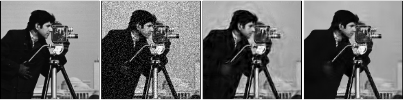
Fig. 7. A fragment of Cameraman . From left to right: original, noisy observation ( \sigma=25 , PSNR=20.14dB), BLS-GSM estimate [42] (PSNR=28.35dB), and the proposed Pointwise SA-DCT estimate (PSNR=29.11dB).
