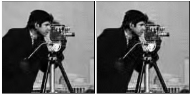
Fig. 21. Denoising of Cameraman ( \sigma=25 , observation shown in Figure 7) using B-DCT with fixed block of size 8 \times 8 (left) and 16 \times 16 (right). The PSNRs of the two estimates are 28.83dB and 28.63dB, respectively. Compare with the Pointwise SA-DCT estimate shown in Figure 7 (PSNR=29.11dB).
