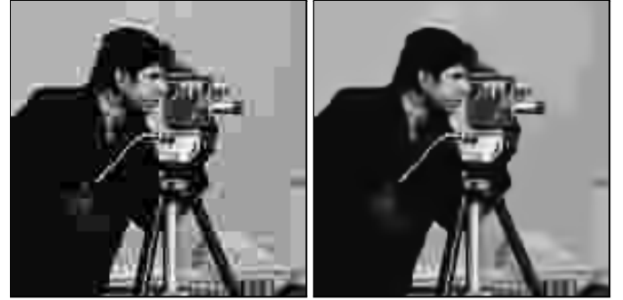
Fig. 9. Details of the JPEG-compressed Cameraman ( Q=6 , \text{bpp}=0.19 , PSNR=25.03dB) and of the corresponding Pointwise SA-DCT estimate (PSNR=26.11dB). The estimated standard deviation for this highly compressed image is \sigma=17.6 .
