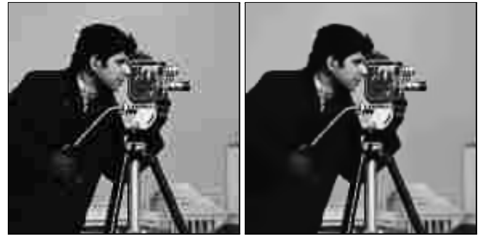
Fig. 10. Details of the JPEG-compressed Cameraman ( Q=15 , \text{bpp}=0.37 , PSNR=27.71dB) and of the corresponding Pointwise SA-DCT estimate (PSNR=28.58dB). The estimated standard deviation for this compressed image is \sigma=9.7 .
