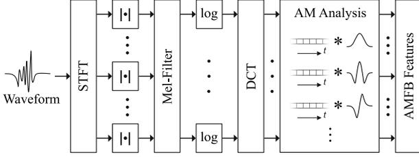
Fig. 1. Signal processing scheme to extract amplitude modulation filter bank features.
