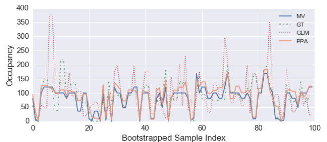
Figure 6: Ground Truth (GT) and predictions using the above described techniques. Poisson Regression (GLM) performs considerably worse than the GMM-HMM models.
