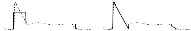
Fig. 1. A feature of an example signal as a function of time (dashed lines) and the density means of the optimal state transition paths of a hidden Markov model (solid line, left plot) and the proposed model (solid line, right plot).
