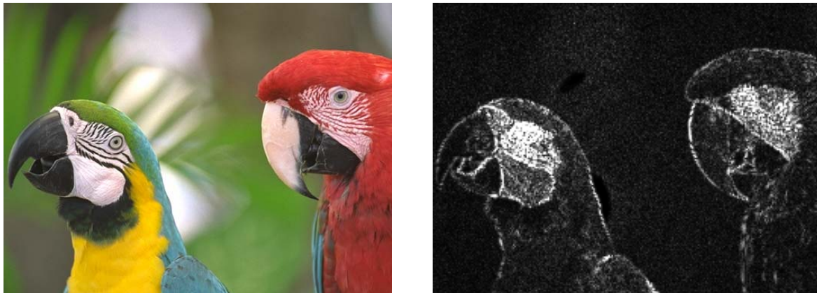
Fig. 3. Portrait photography mode image and zoomed local power map for its Y component (lighter pixels correspond to larger values of E_{ij} )
