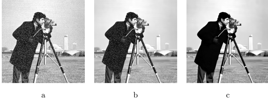
Figure 7: Complex-valued test image 16: a) noisy phase, b) phase reconstruction by PhAm-BM3D, PSNR_{\varphi}=39.6 dB, c) phase reconstruction by ImRe-BM3D, PSNR_{\varphi}=45.7 dB.
