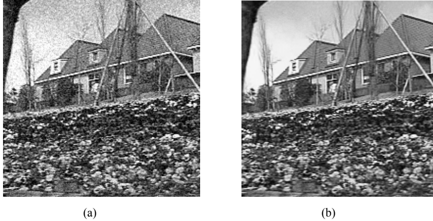
Fig. 4. A fragment of the 30 th frame of the “Flower” video sequence. (a) Noisy (PSNR of fragment 22.41dBs). (b) Denoised with the proposed algorithm (PSNR of fragment 26.39 dBs)
