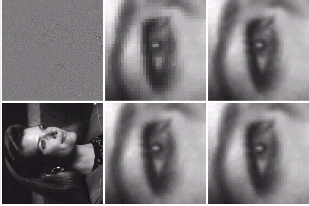
FIGURE 8.34 Approximations of Fig. 8.23 using 25% of the DCT coefficients: (a) and (b) 8 \times 8 subimage results; (c) zoomed original; (d) 2 \times 2 result; (e) 4 \times 4 result; and (f) 8 \times 8 result.
