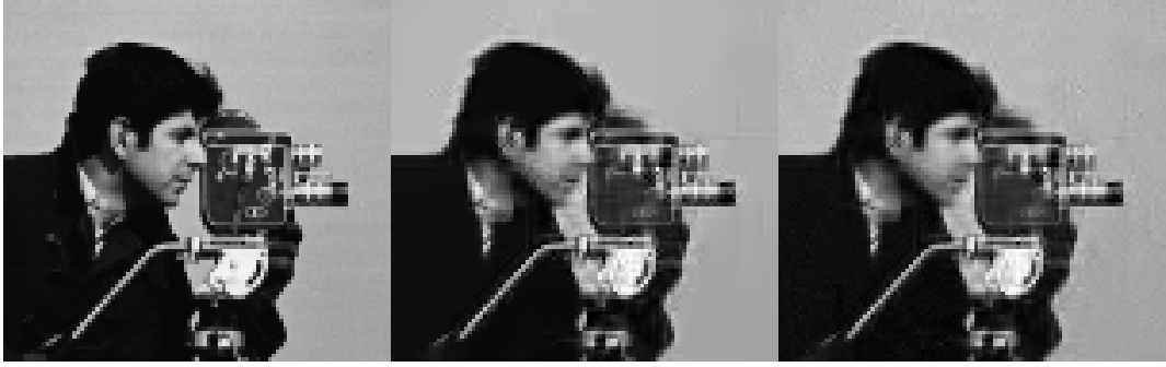
Figure 1: Fragment of the cameraman test-image, \sigma = 25 : true image (left); novel algorithm, PSNR = 29.30 dB (middle); basic thresholding BM3D algorithm PSNR = 29.01 dB (right).
