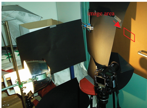
Fig. 2. Measurement setup at TUT/ASE. Image shot with flashlight. One cardboard sheet (attached to stand) is used as a screen to form shadow in target area (brightly illuminated). Others are to prevent disturbing reflections from walls, furniture and miscellaneous laboratory equipment.
