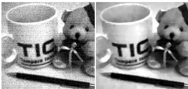
Figure 4: Raw data from cameraphone's CMOS sensor, R channel, 1ms exposure (left), and reconstructed image using the LPA-ICI adaptive method with the estimated variance function.
