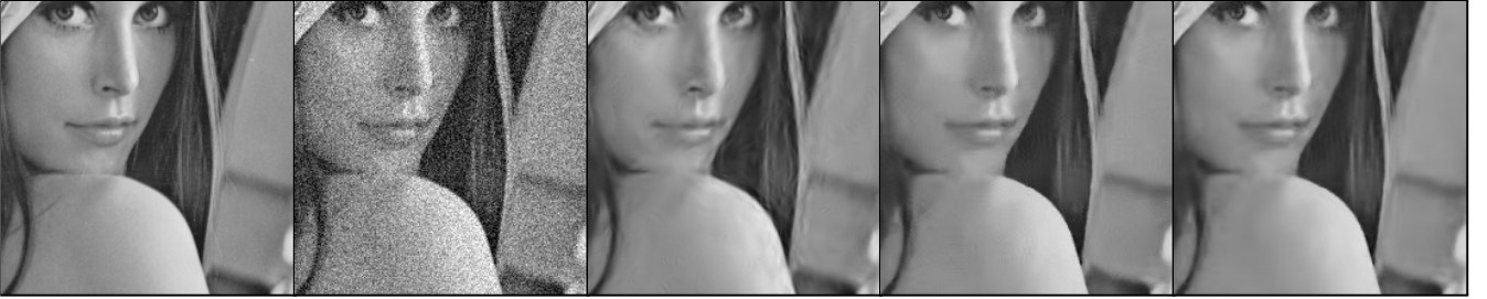
Figure 6: A fragment of Lena . From left to right: original image, noisy observation ( \sigma=25 ), GSM estimate [22] ( PSNR=31.69 dB), and Anisotropic LPA-ICI SA-DCT estimates \hat{y} (7) and \hat{y}^{wi} (10) ( PSNR=31.24 and 31.65 dB, respectively).
