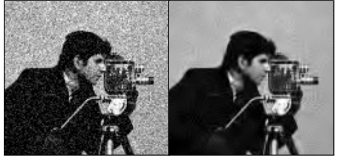
Figure 4: Cameraman : noisy observation ( \sigma=25 ), and sliding 8 \times 8 block DCT estimate ( PSNR=28.36\text{dB} ).
