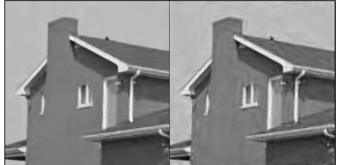
Figure 7: House : two estimates obtained from the same noisy observation (not shown) with \sigma=25 : (left) the Anisotropic LPA-ICI SA-DCT Wiener estimate, PSNR=31.92 dB, and (right) the GSM estimate [22], 31.40 dB. The PSNR of the reference estimate (7) is 31.55 dB.
