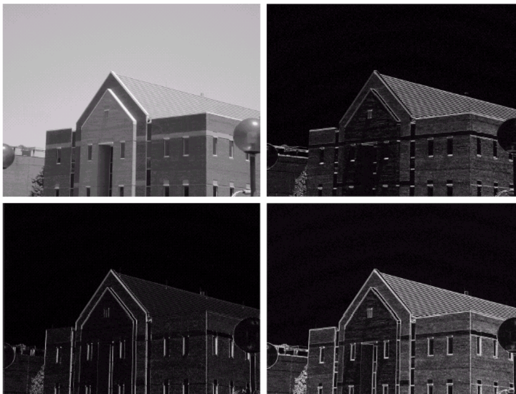
FIGURE 10.10 (a) Original image. (b) |G_x| , component of the gradient in the x -direction. (c) |G_y| , component in the y -direction. (d) Gradient image, |G_x| + |G_y| .
