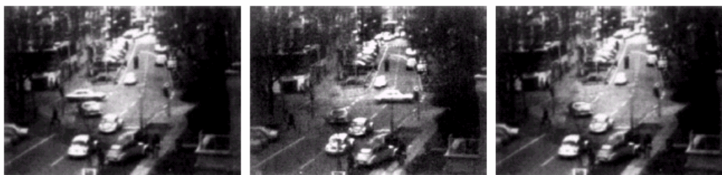
FIGURE 10.50 Building a static reference image. (a) and (b) Two frames in a sequence. (c) Eastbound automobile subtracted from (a) and the background restored from the corresponding area in (b). (Jain and Jain.)
