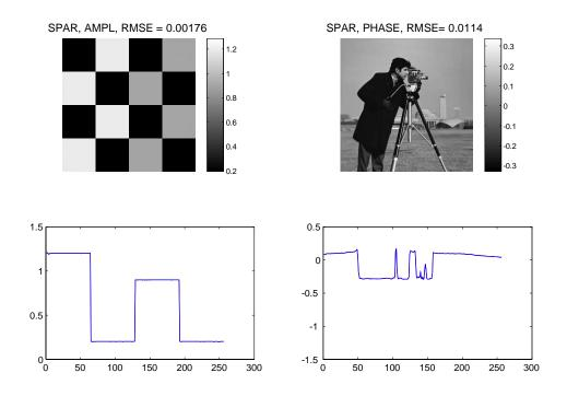
Fig. 4. The amplitude modulation by the binary chessboard test-image and the phase modulation by the gray-scale cameraman test-image, noiseless data. The reconstruction by the proposed SPAR algorithm. The visual quality of the reconstructions is almost perfect. In the cross-sections a di¤erence between the true signal and the reconstructions is slightly seen only in the phase reconstruction.
