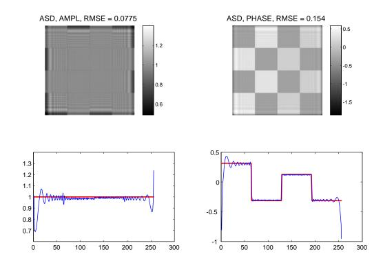
Fig. 1. The phase modulation object with the binary phase (chessboard testimage), noiseless data. The reconstruction by the ASD algorithm. In the cross-sections thick ('red' in color) and thin ('blue' in color) lines show the true signal and the reconstructions, respectively. RMSE values for the phase and amplitude are shown at the top. The visual quality of the reconstruction is quite poor: wiggles, waves, etc. are clearly seen.
