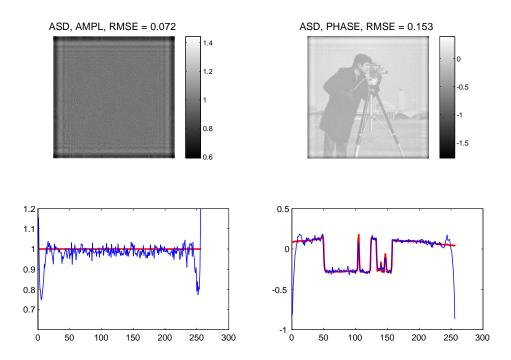
Fig. 5. The phase modulation by the gray-scale cameraman test-image, noisy data. The reconstruction by the ASD algorithm. In the cross-sections thick ('red' in color) and thin ('blue' in color) lines show the true signal and the reconstructions, respectively. The visual quality of the reconstructions is poor: artifacts and noise are well seen.
