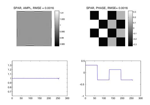
Fig. 2. The phase modulation object with the binary phase (chessboard testimage), noiseless data. The reconstruction by the proposed SPAR algorithm. The visual quality of the reconstruction is perfect: wiggles, waves and other artifacts are completely wiped out. In the cross-sections the di¤erence between the true signal and the reconstructions is not seen.
