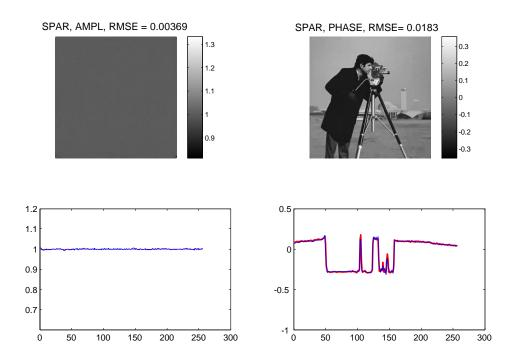
Fig. 6. The phase modulation by the gray-scale cameraman test-image, noisy data. The reconstruction by the proposed SPAR algorithm. RMSE values for the phase and the amplitude are shown at the top. The visual quality of the reconstruction is quite good: wiggles, waves, other artifacts and noisy are nearly wiped out. The noise level in the reconstructions is quite low in comparison with what is achieved in Fig.5.
