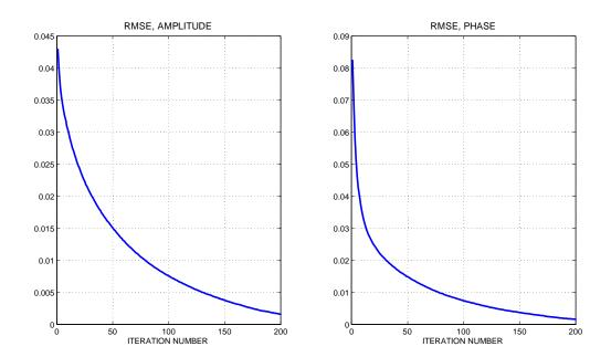
Fig. 7. RMSE for the amplitude and phase reconstructions by the proposed SPAR algorithm versus the number of iterations. The phase modulation object with the binary phase (chessboard test-image), noiseless data.
