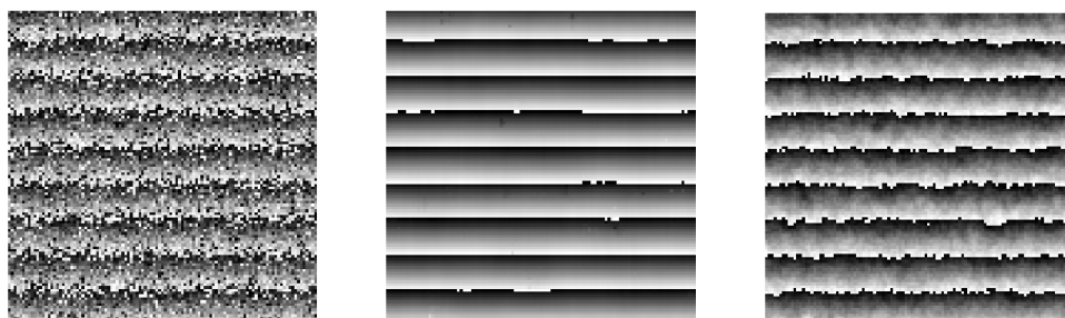
Fig. 4. Wrapped Ramp phase: a) noisy, b) PhaseLa rewrapped, c) Z\pi M rewrapped.
