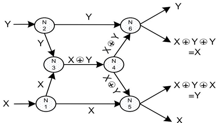
Fig. 1. Example of network coding in multicasting scenario.
