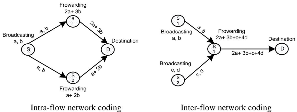
Fig. 4. Example of intra-flow and inter-flow network coding.
