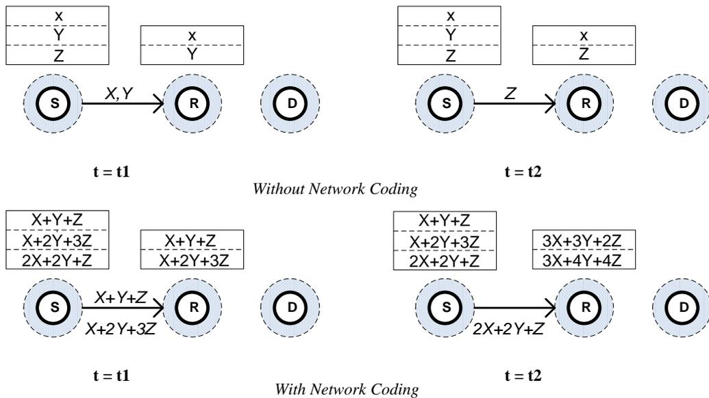
Fig. 3. Improving buffer performance using network coding.
