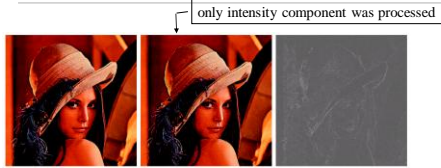
FIGURE 6.41 Image sharpening with the Laplacian. (a) Result of processing each RGB channel. (b) Result of processing the intensity component and converting to RGB. (c) Difference between the two results.
