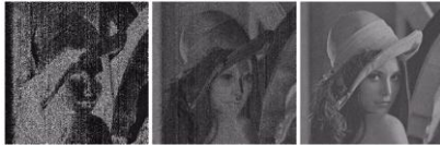
FIGURE 6.49 HSI components of the noisy color image in Fig. 6.48(d). (a) Hue, (b) Saturation, (c) Intensity.
