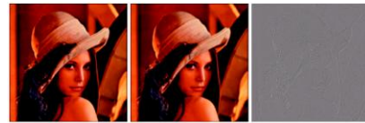
FIGURE 6.40 Image smoothing with a 5 \times 5 averaging mask. (a) Result of processing each RGB component image. (b) Result of processing the intensity component of the HSI image and converting to RGB. (c) Difference between the two results.
