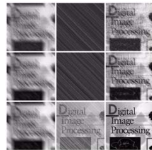
FIGURE 5.29 (a) Image corrupted by motion blur and additive noise. (b) Result of inverse filtering. (c) Result of Wiener filtering. (d)-(f) Same sequence but with noise variance one order of magnitude less. (g)-(i) Same sequence but with noise variance reduced by five orders of magnitude from (a). Note in (d) how the deblurred image is quite similar to the original image.
