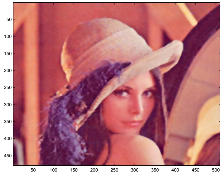
Figure 5: Interpolated image using the separable rational filter from the (1/16) rectangular decimated image.
