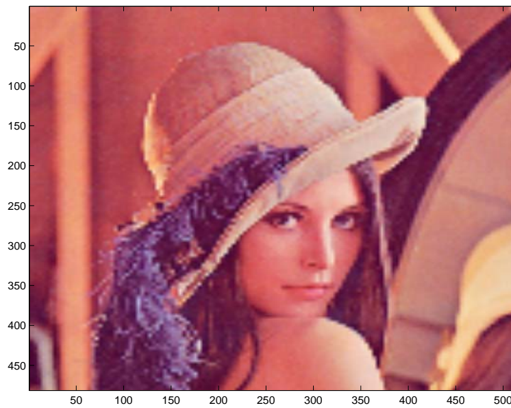
Figure 3: Interpolated image using the vector median hybrid filter from the (1/16) rectangular decimated image.
