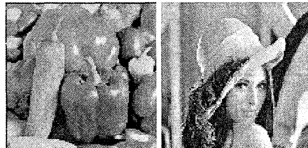
Fig. 5. Image filtered by Spline fitting with covariance matrix unknown, PSNR = left : 24.87dB, right : 22.49dB.
