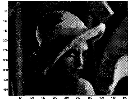
Figure 6: Interpolated image by the bidirectional algorithm using the vector rational filter from the (1/16) rectangular decimated image.
