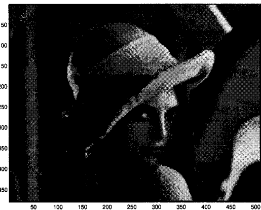
Figure 7: Interpolated image by the mixed algorithm using the vector rational filter from the (1/16) rectangular decimated image.
