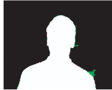
FIGURE 13: The colored segmentation error of frame 15 from the sequence “Erik,” segmented using COST AM 5.0.
