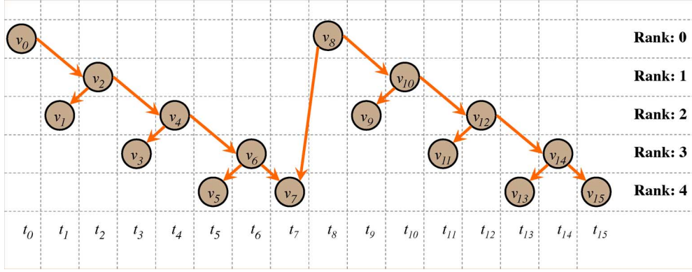
Fig. 4. Hasse diagram describing the poset of access-units, ordered based on decoding precedence, for the graph shown in Fig. 1(b).
