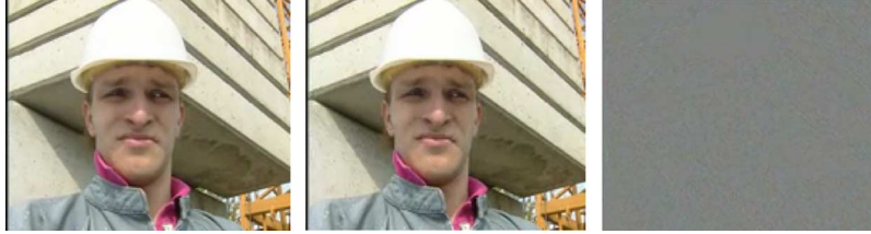
Fig. 5. Sample video splicing results using a quantization parameter of 28 for the both SBS and DRBS, from left to right: spliceable bit stream, spliced bit stream and splicing error after propagated over 14 inter pictures.
