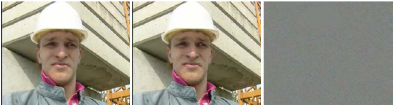
Figure 5: Sample video splicing results using a quantization parameter of 28 for the both SBS and DRBS, from left to right: spliceable bit stream, spliced bit stream and splicing error after propagated over 14 inter pictures
