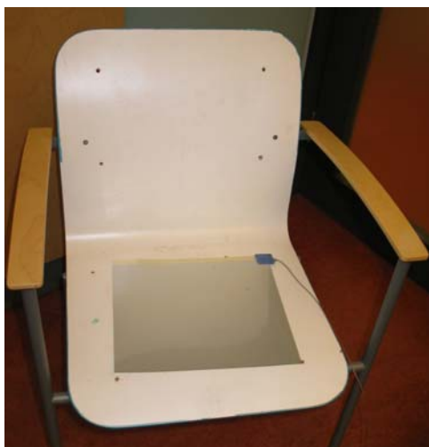
Figure 2. A 27,6 x 30 cm EMFi sensor sheet applied on a chair
