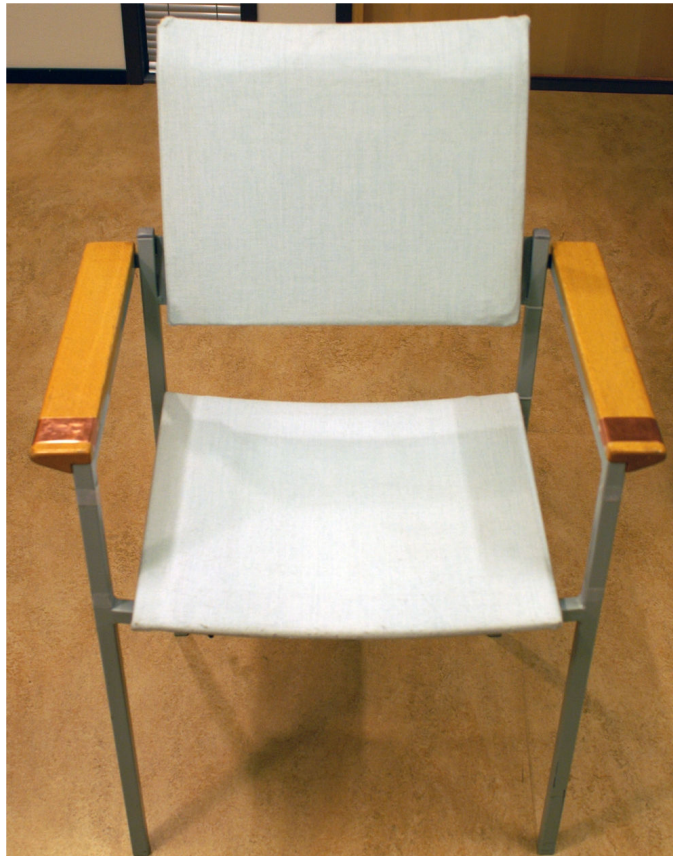
Figure 3. The finished prototype of the ProHeMon chair. The sensors are hidden in the upholstery of the chair and the amplifiers and wireless link electronics are in a box under the seat. The strips of copper on the arm rests serve as ECG electrodes.
