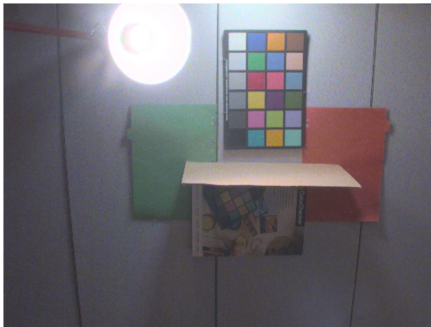
Fig. 21. HDR image composed and tone mapped from the noisy (ISO 800) sequence in luminance-chrominance (opponent) color space.
