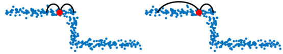
Fig. 1. Adaptive isotropic neighborhoods (left) and adaptive directional neighborhoods (right) indicated by black curved lines for a point (in red) located close to a sharp edge in a 2-D noisy point cloud. Using adaptive directional neighborhoods provides larger supports for a local estimate even when the points are close to sharp features.
