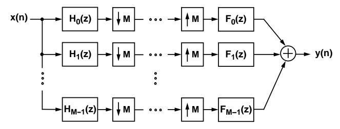
Linear-phase prototype filter:
