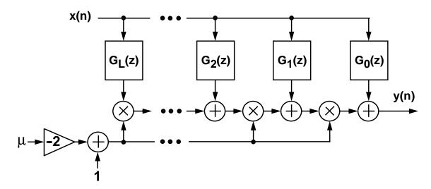
Fixed linear-phase filters for  $l = 0, 1, \dots, L$ :
