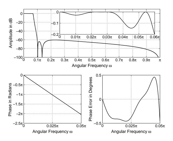
For the optimized filter, only 10 adders with 11 fractional bits are required to implement all the adaptor coefficients.
