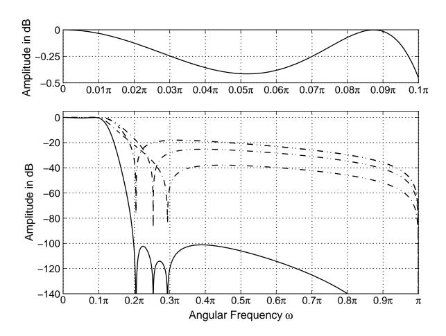
For the cascade of four LWD filters, only **5** fractional bits are needed for coefficient implementation compared to **9** bits required by the direct LWD filter.
