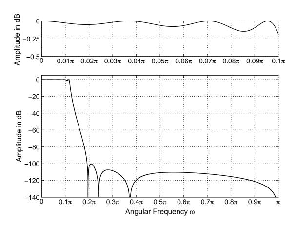
Alternatively, cascade of **four 3rd-order** LWD filters is needed to satisfy the amplitude specifications.
